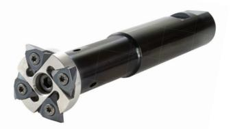
**MT7** Sub-Micron Grade with Titanium Aluminum Nitride multi-layer coating (ISO K10 - K20). This is a general purpose grade, which can be used with all materials; it should be run at medium to high cutting speeds.
